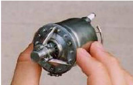
Fig. 6. Stanford/M-DOT gas turbine [23].
