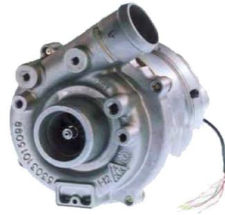
Fig. 4. eBooster from BorgWarner—an electrical power air compressor providing pressurized air for the support of the turbocharger at low engine speeds [19].
